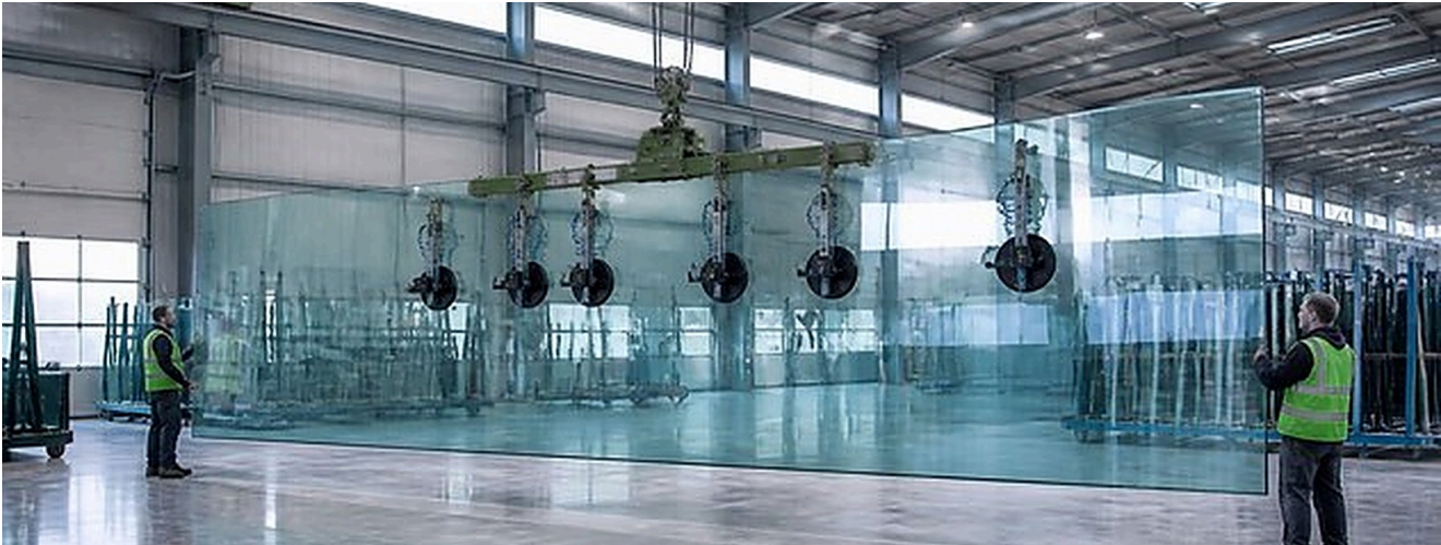
OVERSIZED LITE UNDER VACUUM LIFTER — FACTORY HANDLING
